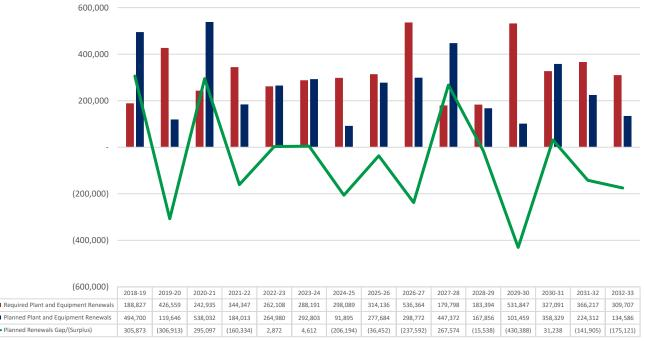
The chart reflects a lack of correlation between the Plant Replacement Program and the estimated useful life of plant and equipment provided by the valuers. The Plan overall has a funding deficit of \$800k over the term of the Plan with planned renewals of \$4.0m and required asset renewals of \$4.8m.
