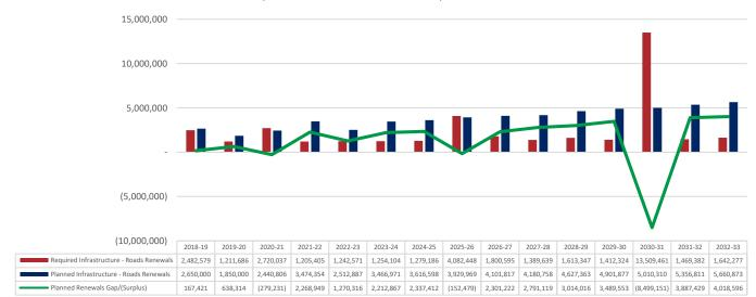
The level and extent of the renewal surplus is dependent on the accuracy of unit cost estimates and remaining useful life estimates for each road component. An improvement in this information will result in improved planning outcomes and enable the scheduling of works to minimise the negative impact of renewal spikes such as occurs in 2030-31.
